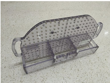
图2 2D几何畸变测量模体 Figure 2 2D geometric distortion measurement phantom
