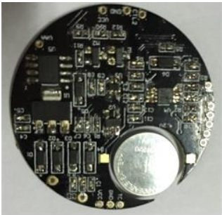
图9 无线能量接收板 Figure 9 Wireless energy receiving board
