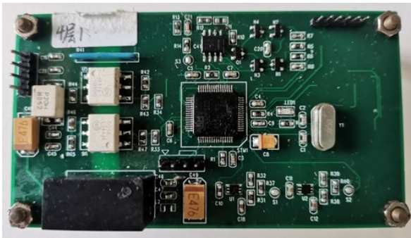
图9 自适应脉搏氧板卡 Fig.9 Circuit board of adaptive pulse oximetry
