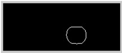
图23 筛选出瞳孔边缘 Fig.23 Outlined pupillary edge
