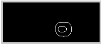
图22 边缘检测后瞳孔 Fig.22 Pupil after edge detection
