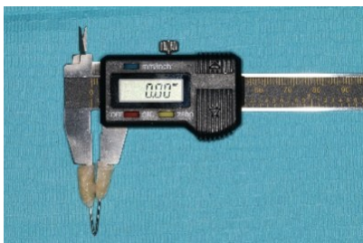
图6 改良测量尺 Fig.6 Improved measuring scale
