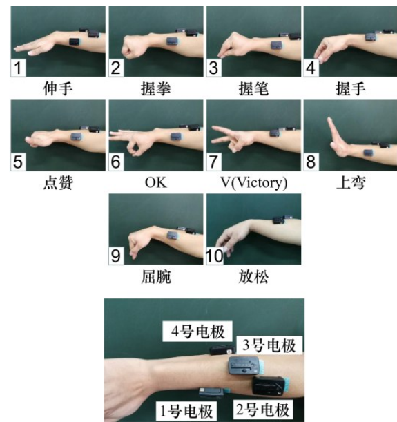
图4 手势动作及电极安装位置 Fig.4 Hand gestures and electrode installation positions
