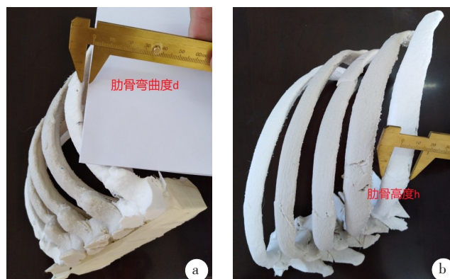
图2 3D打印模型进行体外测量肋骨处高度 h 值及弯曲度 d 值 Fig.2 In vitro measurements of the height (Fig.a) and curvature (Fig.b) of 3D printed model
