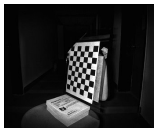
b: IR camera calibration
