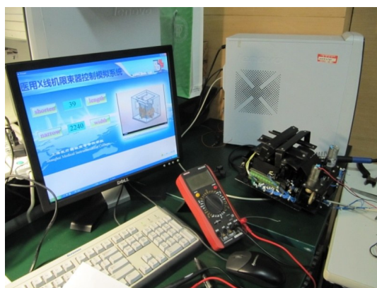
图7 X线机限束器控制系统软件界面 Fig.7 Software interface of X-ray collimator control system
