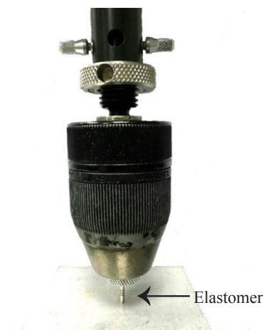
图6 压缩实验装置图 Fig.6 Experimental set-up of compression
