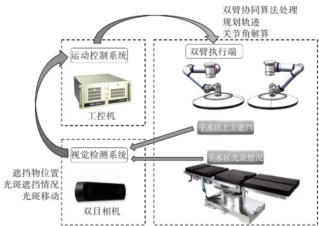
图2 智能双臂无影灯系统构成示意图 Figure 2 Schematic diagram of the composition of the intelligent dual-arm shadowless lamp system
