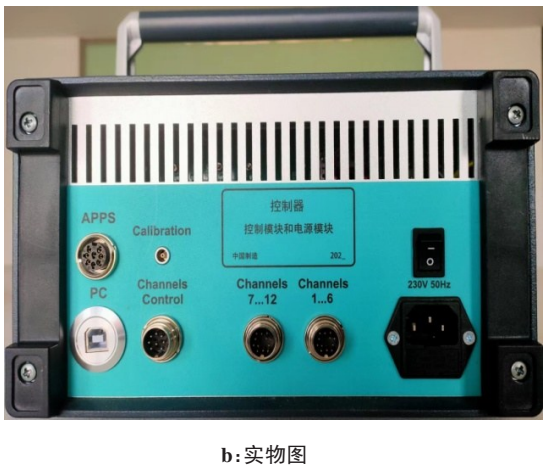
图 2 主机控制器电路 Figure 2 Circuit structure of the host controller
