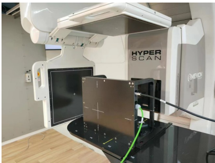
图3 90°机架角下模体摆位示意图 Figure 3 Diagram of the phantom setup as gantry at 90°
