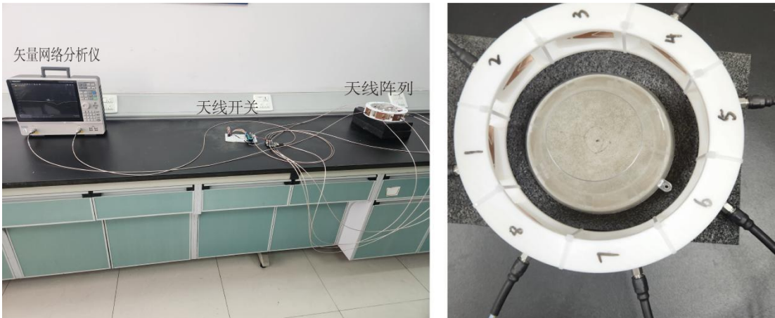
图6 模拟实验装置 Figure 6 Simulation experimental devices
