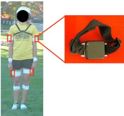
图1 基于惯性传感器的爬行运动数据采集系统 Figure 1 A crawling motion data acquisition system designed based on inertial sensors
