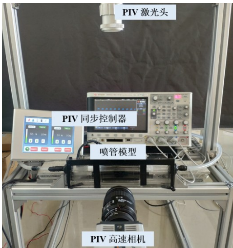
图 11 PIV 实验系统与模型 Figure 11 PIV experimental system and model
