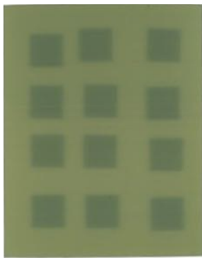
图3 整张胶片测试不均匀性实际照射结果 Figure 3 Actual irradiation results for testing non-uniformity across the whole film
