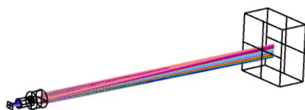
图2 Zemax 模拟的光学成像系统模型示意图 Figure 2 Schematic diagram of the optical imaging system model simulated by Zemax
