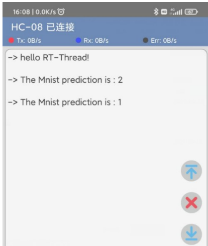
图6 蓝牙调试器接收的预测信号 Figure 6 Predictive signal received by Bluetooth debugger
