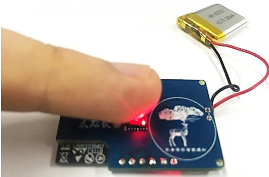
图2 PPG信号采集过程示意图 Figure 2 PPG data acquisition process
