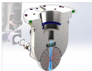
图3 Zap-X系统旋转式辐射准直器 Figure 3 Rotary collimator of Zap-X system
