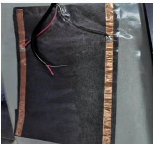
图3 一片碳纤维导电加热片 Fig.3 A slice of carbon fiber conductive heating plate
