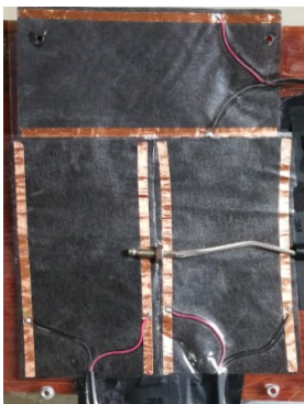
图4 组合而成的大加热片 Fig.4 Composed heating plate
