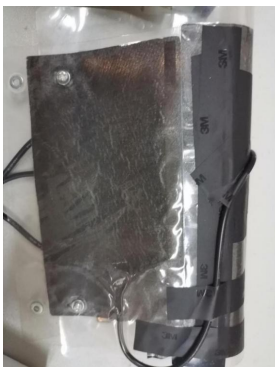
图5 螺丝固定的包围加热体 Fig.5 Screw-mounted enclosing heater
