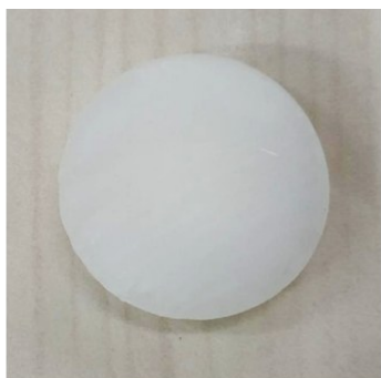
图3 压缩测试试样 Fig.3 Compression test sample
