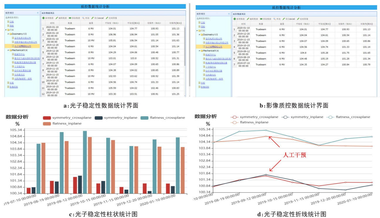
图2 QAManager数据统计界面 Fig.2 QAManager interfaces for data statistics
