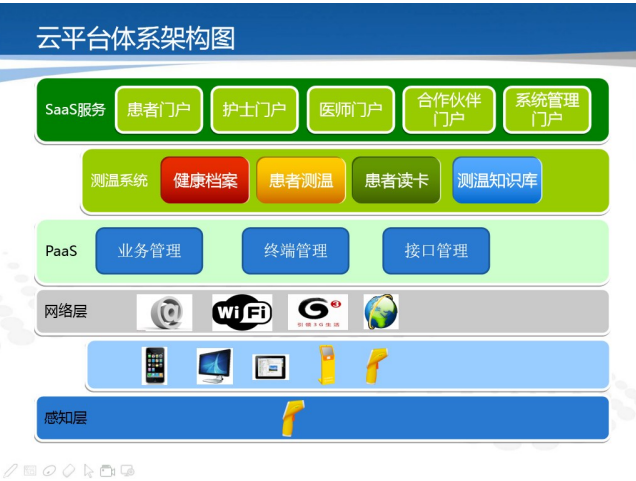
图4 云平台体系架构图 Fig.4 Cloud platform architecture diagram
