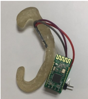
图2 耳后脉搏信号检测系统 Fig.2 System for detecting the pulse signals behind the ear
