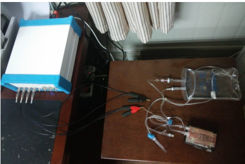
图4 利用阻抗分析仪采集流动液的电阻抗数据 Fig.4 The PFL's impedance data collected by using an impedance analyzer
