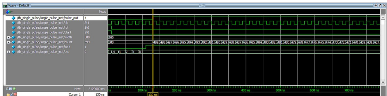
图13 单脉冲上升沿仿真 Fig.13 Simulation of monopulse rising edge
