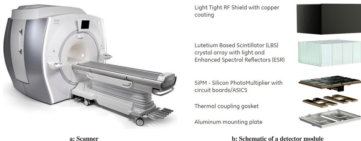
图5 通用电气全身PET/MRI成像系统 Fig.5 The whole body PET/MRI scanner developed by GE
