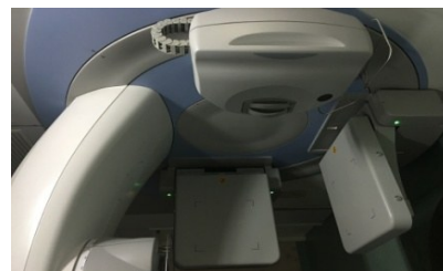
图1 医科达Synergy Platform加速器及所载CBCT设备 Fig.1 ELEKTA Synergy Platform accelerator and cone beam computed tomography (CBCT) device
