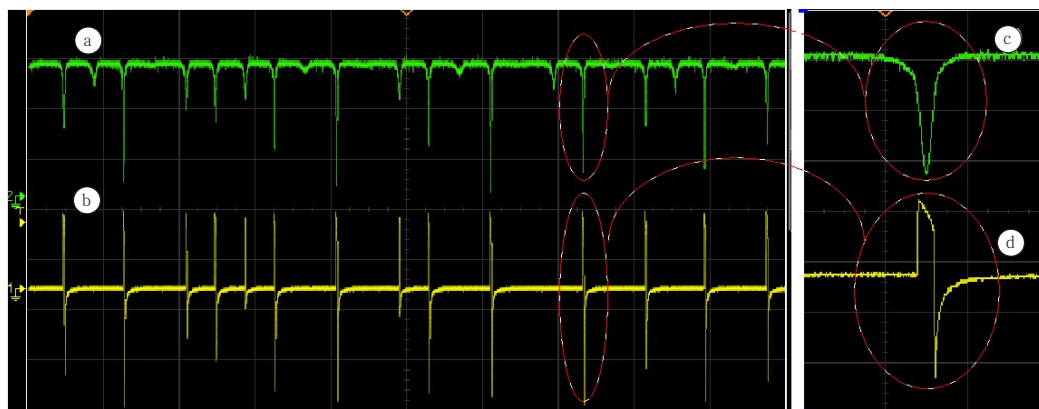
a: Transformed z(t) signal; b: Bipolar asymmetric pulse wave; c: Amplified detail signal of Fig. 4a; d: Amplified detail signal of Fig. 4b
