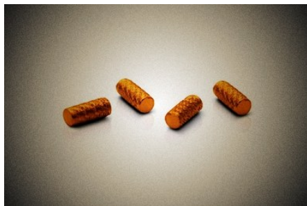
The diameter of gold seed is 0.8 mm, with a length of 4.0 mm.
