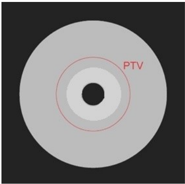
The value of the density of this phantom is 1.0 in the dark grey area, 0.9 in the light grey area and 0 in the dark area.
