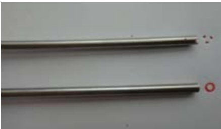
图1 点触式探针与平面探针照片 Fig.1 Point contact probe and plane probe The upper one is a point contact probe. The down one is a plane probe
